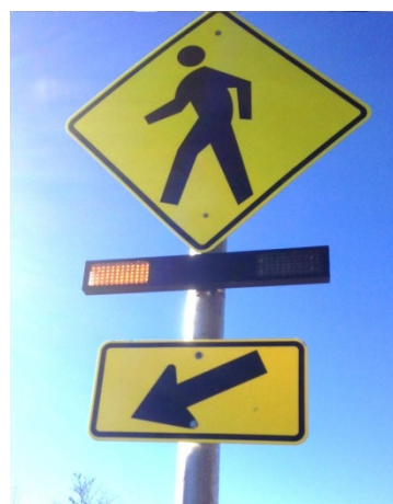
Figure 29. Rectangular Rapid Flashing Beacon
