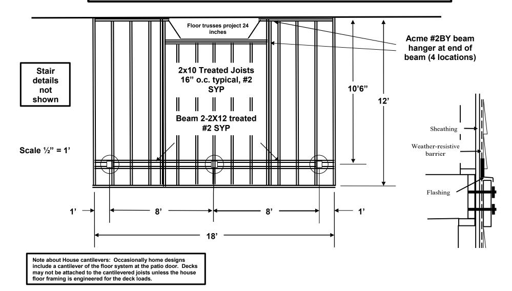
WARNING: THIS IS AN ILLUSTRATION ONLY. IT IS INTENDED TO SHOW SOME OF THE INFORMATION THAT SHOULD BE INCLUDED ON YOUR DECK PLANS. IT IS <u>NOT</u> INTENDED TO SHOW COMPLIANCE WITH ANY CODES THAT MAY APPLY. CHANGES IN THE HEIGHT AND SIZE OF A DECK WILL CAUSE VARIATIONS IN CODE REQUIREMENTS.
