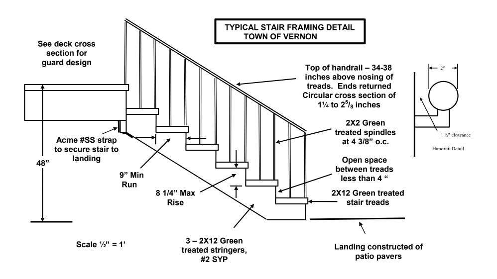
WARNING: THIS IS AN ILLUSTRATION ONLY. IT IS INTENDED TO SHOW SOME OF THE INFORMATION THAT SHOULD BE INCLUDED ON YOUR DECK PLANS. IT IS <u>NOT</u> INTENDED TO SHOW COMPLIANCE WITH ANY CODES THAT MAY APPLY. CHANGES IN THE HEIGHT AND SIZE OF A DECK WILL CAUSE VARIATIONS IN CODE REQUIREMENT.
